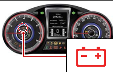
Charge warning lamp on instrument cluster
